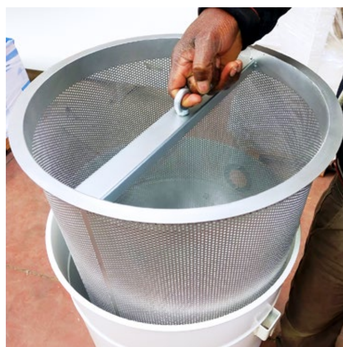
Liquids and solids separator
