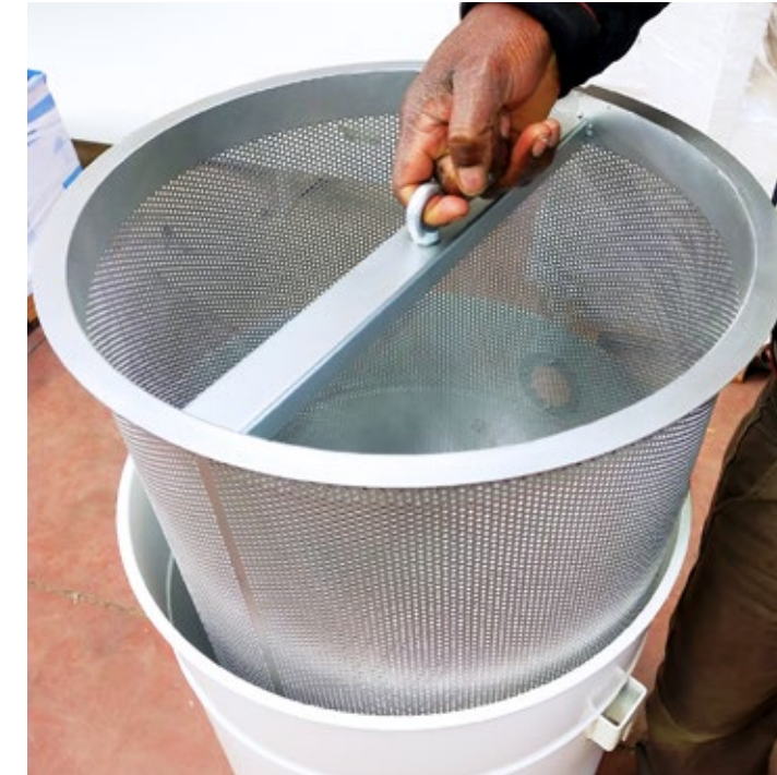
Liquids and solids separator
